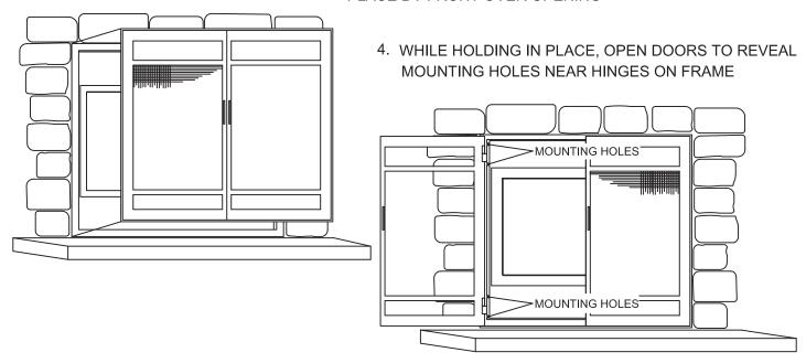
5. USE A PENCIL TO MARK HOLE LOCATIONS THROUGH HOLES AND ONTO OUTER FRAME OF THE FIREPLACE.
